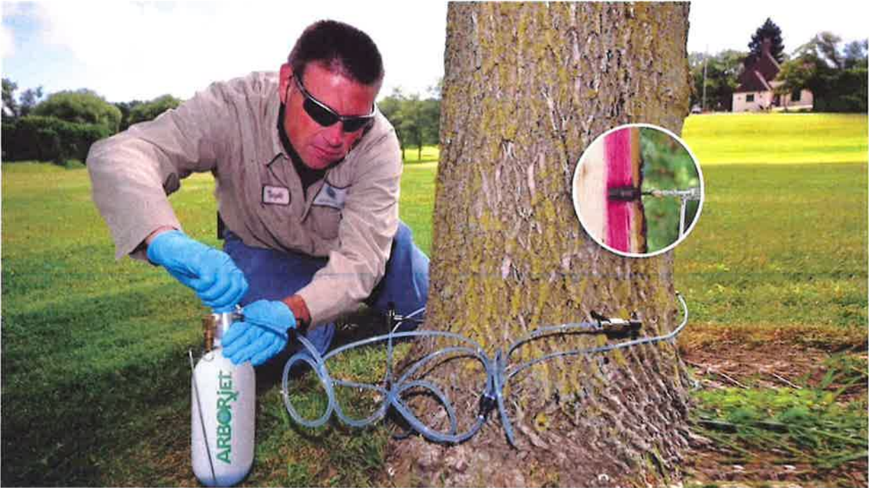
Image 4. Image of Arborjet trunk injection system. Screenshot captured by John O'Neill from perennialgreenlawn.com on May 17, 2022.
